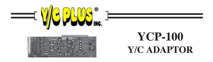
By the addition of the YCP-100 to one of the Amiga Computer's Zorro (Expansion) Slots, the Video Toaster and Flyer system is now converted to true Y/C (S-Video) in and out. The (4) four inputs are parallel with the Video Toaster Inputs. The YCP-100 offers (2) two program Y/C outputs. The preview out remains the composite video output from the Toaster.
