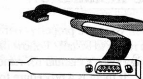
Figure 2.6 - Ribbon cable and bracket assembly (with alternate slot cover plate).
