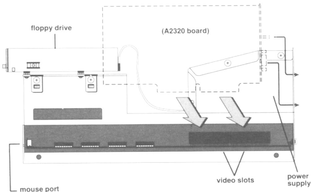
**Fig. 5: A2320 - Installation, Right side View**
