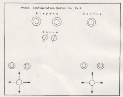
This screen enables you to see if your Fire buttons, Player buttons, coin mechanisms, joysticks and configuration button are all working correctly. Each control flashes green when activated (except the coin mechanisms, which register coin drops). Intermittent or "sticky" buttons can be identified, and joysticks can be fine-tuned for good 8-way response, and to allieviate joystick "bounce".
