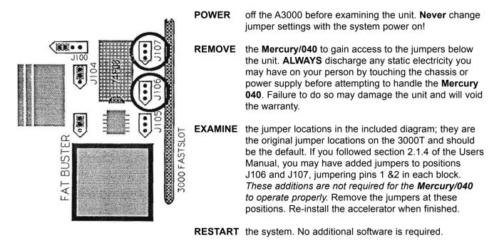
NOTE: Some users have taken to changing jumpers other than what we've suggested. This may change internal system timings that can lead to lockups, non-validated harddisks and floppies and complete systemwide failures. PP&S strongly suggests that you restore the jumpers to the default settings (as in the diagram) before serious data failure occurs.
