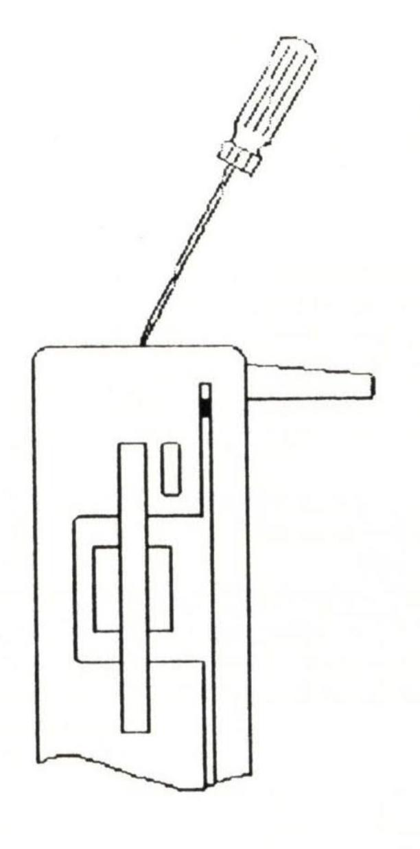
Figure 2: Removing the Amiga's top cover
