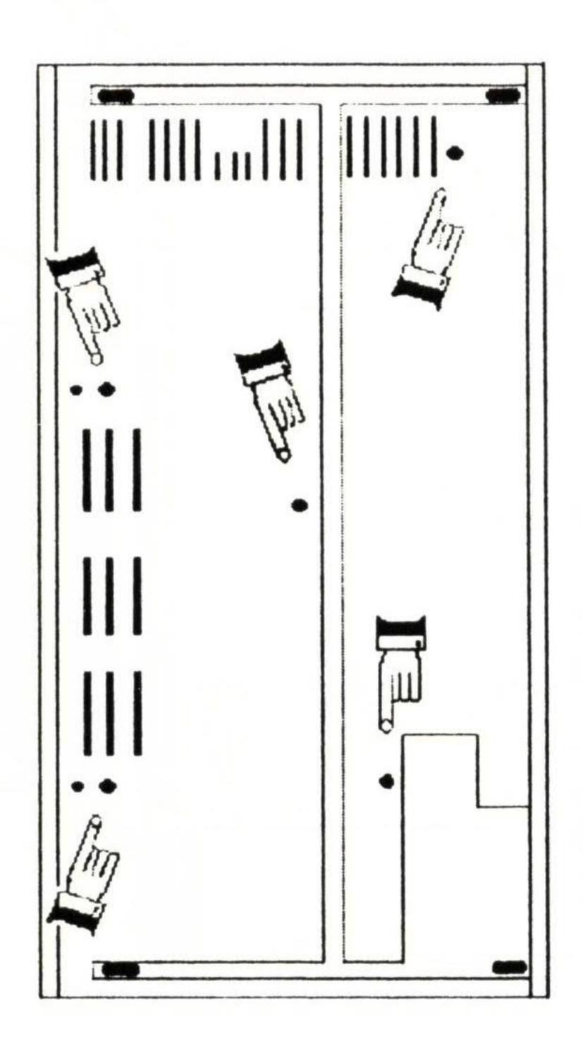
The bottom of the Amiga, showing locations of the top cover screws Figure 1:
