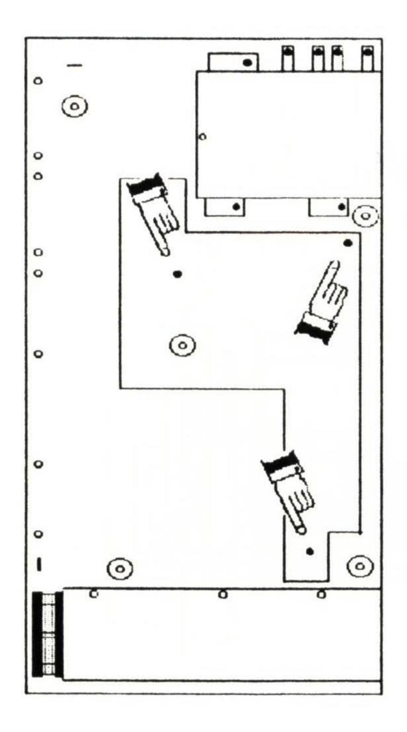
The Amiga with metal shielding removed, showing locations of WCS board screws Figure 4:
