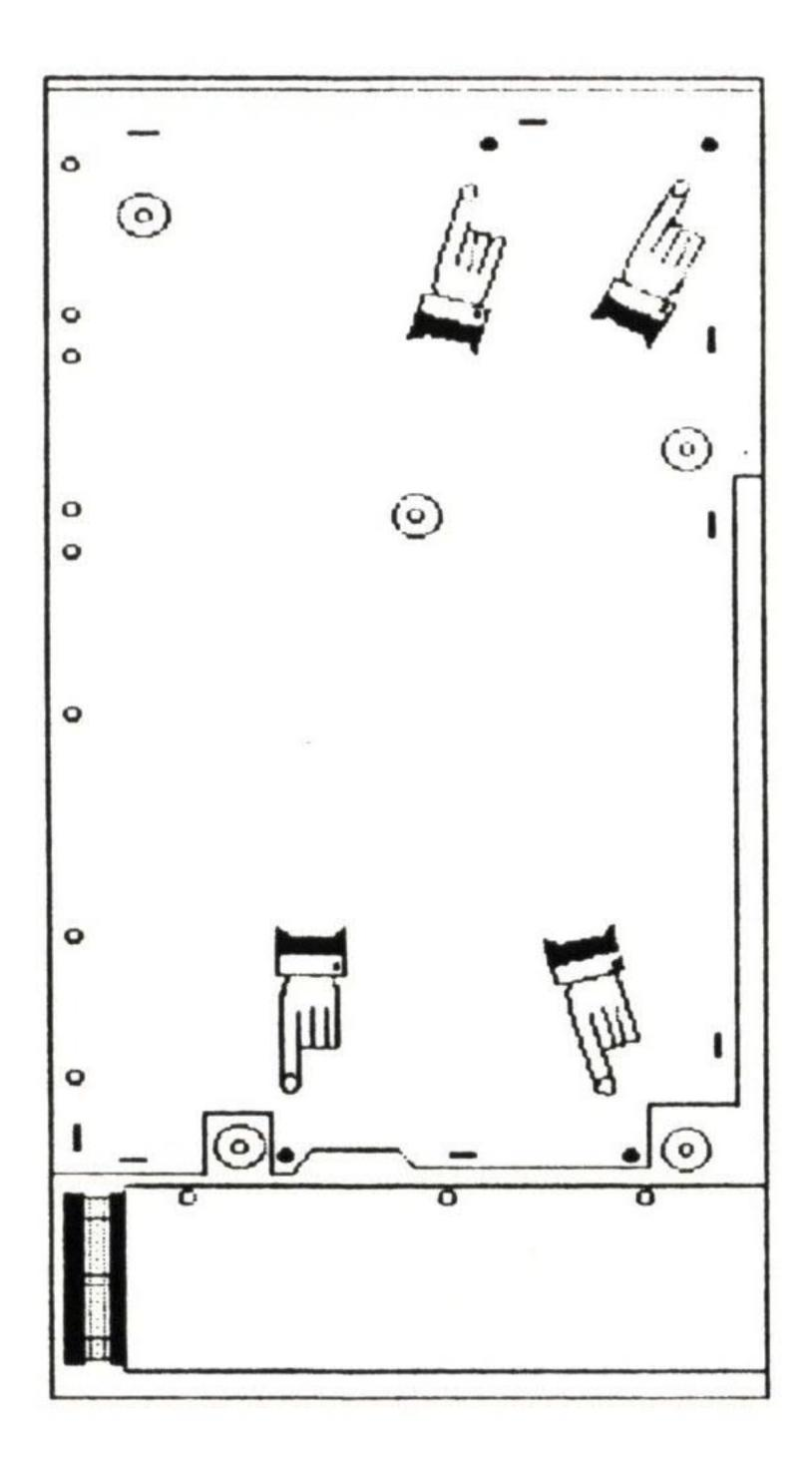
The Amiga with WCS board and internal drive removed, showing locations of main circuit board screws Figure 6:
