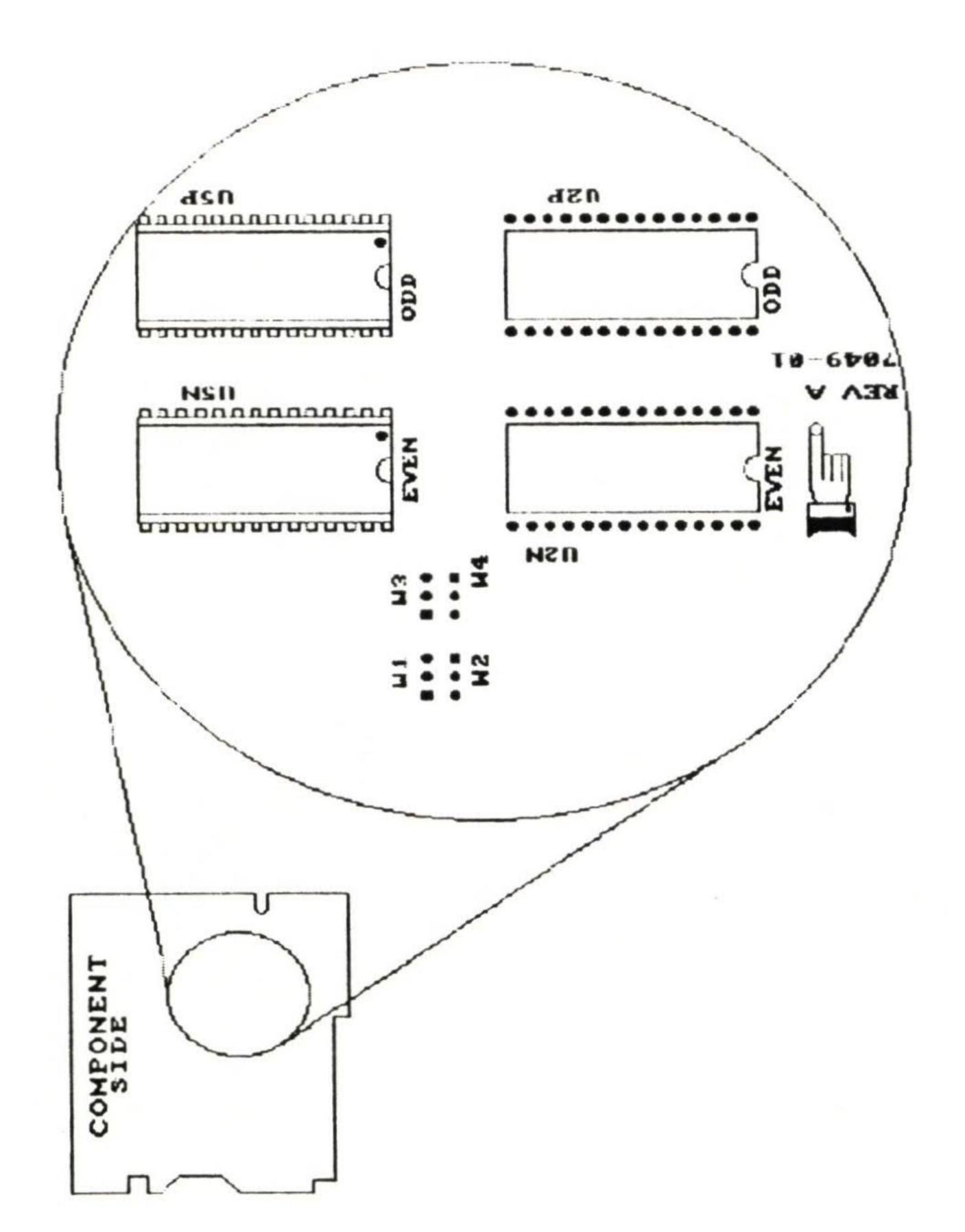
Details of the main circuit board, showing the location of the ROM chips and jumpers Figure 7:
