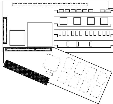
9. Remove the cover plate of a chosen slot, where you would like to insert the connector module. The cover plate is held on by one screw. To make later operations easier, remove the screw completely, even if you can remove the cover plate it only partly unscrewed. Attach the connector module cover plate with the screw that you removed from the empty slot.
