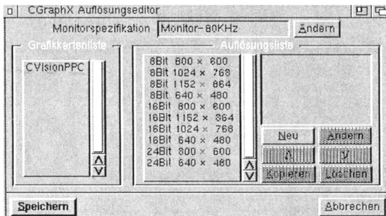
This program produces its own monitor definition files. It is divided into two sections. The first section defines the threshold values of the monitor and the second configures the resolution. Activate the "Monitor Specification" icon to open the window for defining the monitor threshold values.
