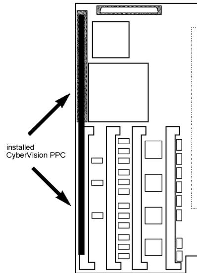
CyberVision PPC is plugged onto the CYBERSTORM MKIII/PPC as shown in picture 5 and 6. In these computers the isolator is not needed.
