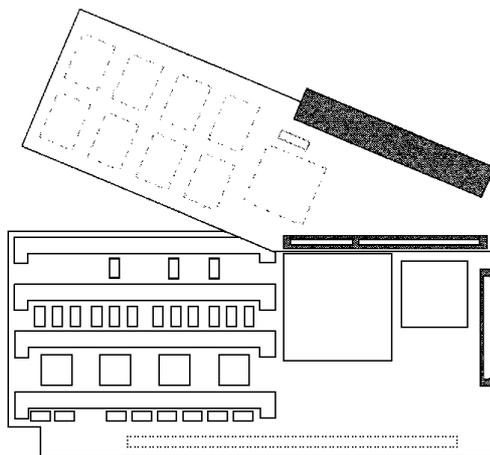
8. Press the card into the slot by pressing on the top of the card. If the CyberVision PPC has been correctly fitted, the connector of the CyberVision PPC and the connector of of
