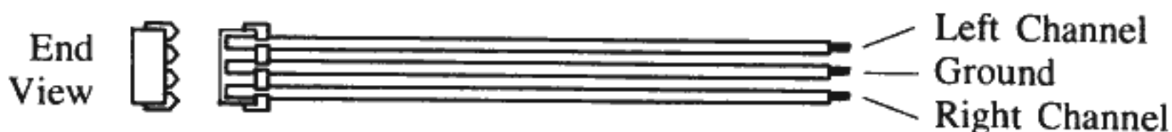
Fig. 10 - CDx-650I Audio Cable Specs
